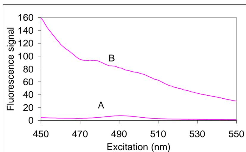
**Figure 2:** Comparison of the synchronous scanning spectra of a uranine standard solution 0,01 ppb (A) and a spring blank sample (B).
