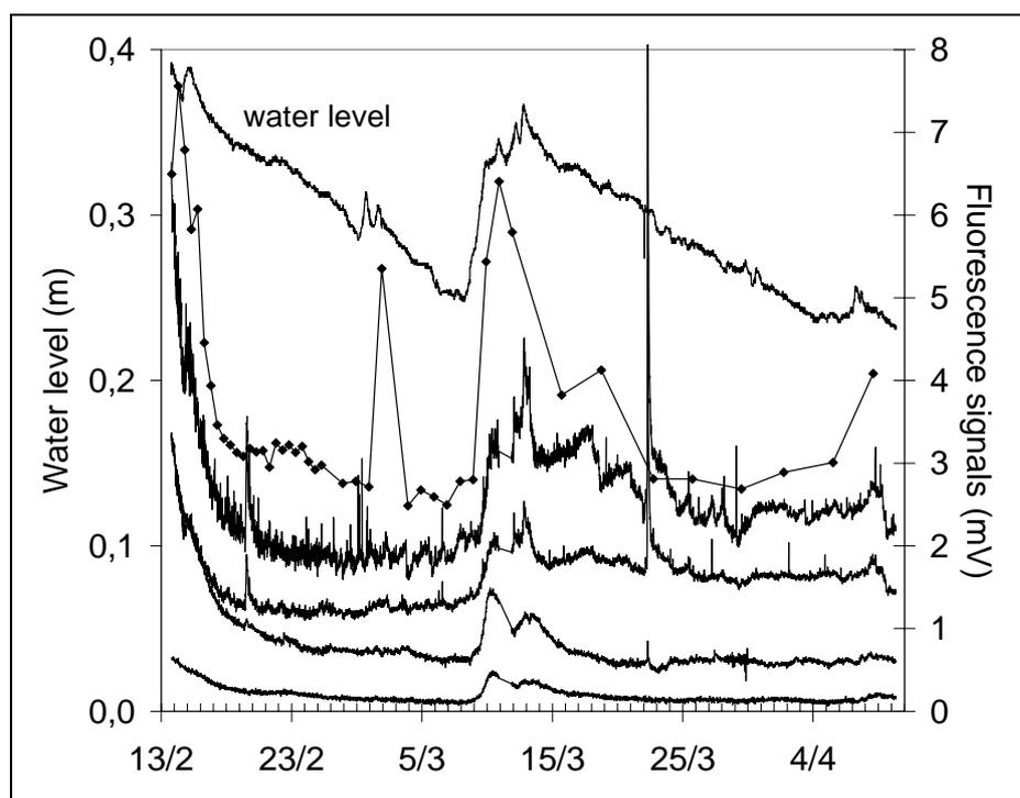
**Figure 10:** Example of monitoring in situ of a karst spring. From top to bottom, the lines are corresponding to: the water level, the fluorescence at 491/511 nm measured by spectrofluorimetry on water samples, the turbidity, the fluorescences measured with the flow-through fluorometer with LEDs at 525, 470 and 370 nm.
