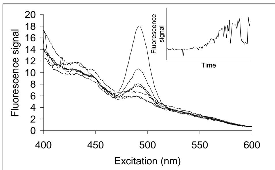
**Figure 9:** Example of the combined use of time serie and synchronous scanning spectra for the demonstration of uranine in groundwater.
